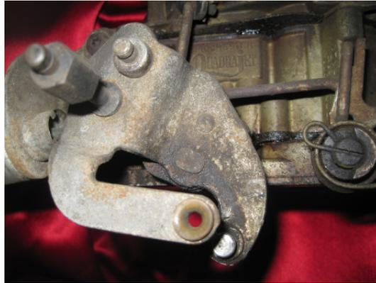
1. Grind the mushroomed retaining flare off the donor shaft and remove the throttle arm from the shaft. **Note** the rectangular keyhole that indexes the arm properly on the shaft.
